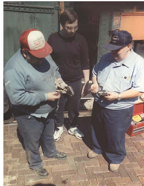
CNS&M 715 getting new inserts in the trolley shoes as the car is readied for the season on the member's work day.
