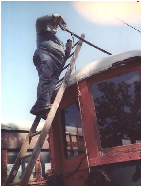
Putting the "trolley shoe" on the "trolley pole" of CNS&M 715.
