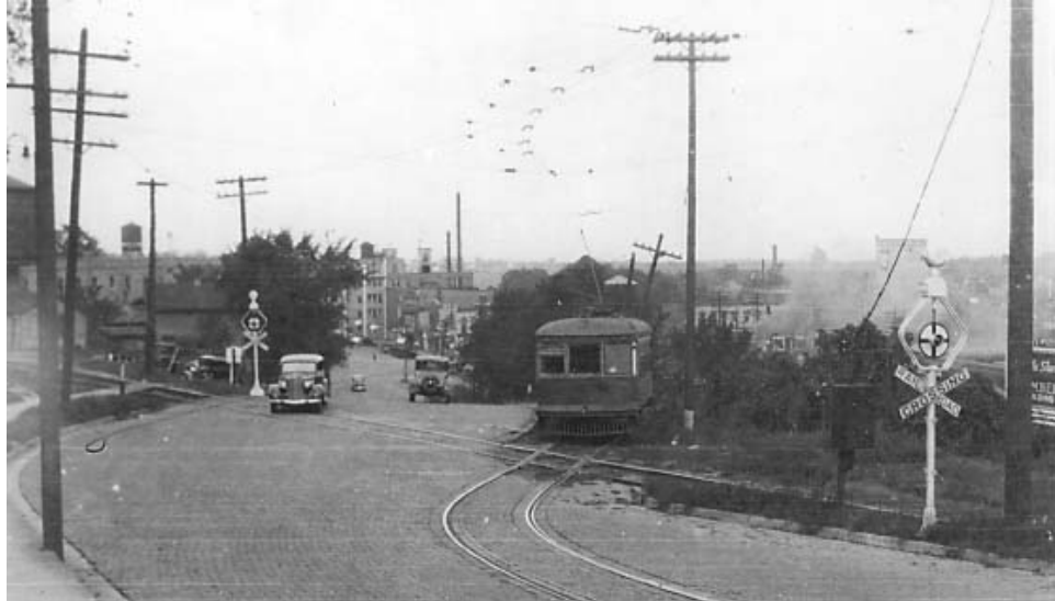
A southbound AE&FRE car near the top of the hill headed for Aurora. Note the C&NW "wig-wag" signal protecting the crossing.
