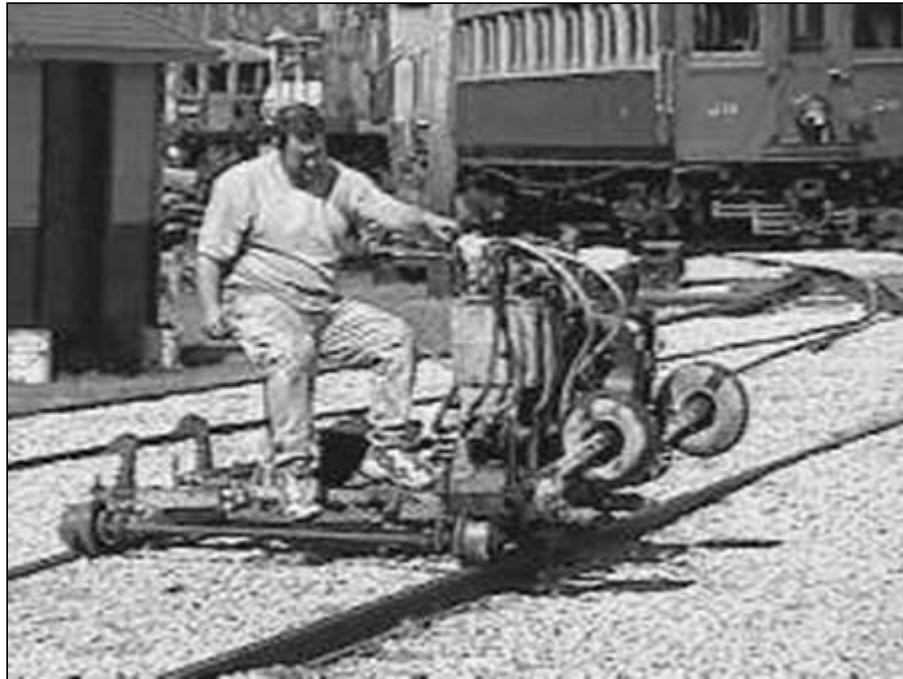
John Sturtz testing our tie inserter prior to it being placed in service. The Inserter is playing a major role in our track rehab program.
