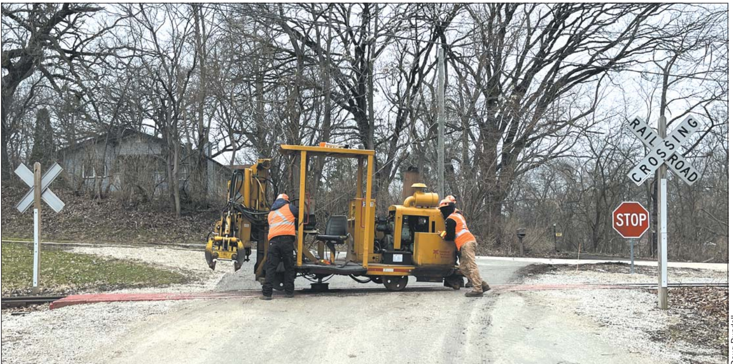
Volkmann crew getting the production tamper on the rails on April 4 th , 2022.
