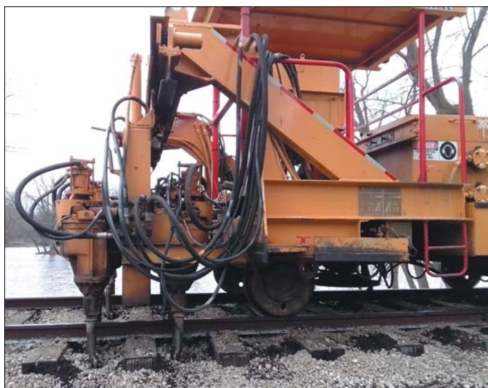
The production tamper at work, tamping every tie in place.
