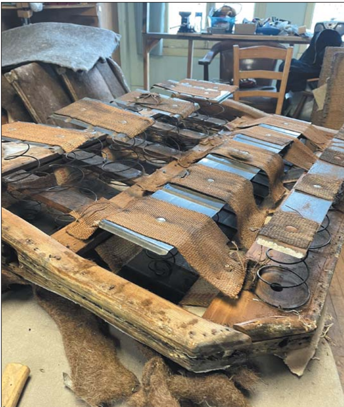
At the shop, a seatback with the old rattan removed exposing wood and webbing defects.
