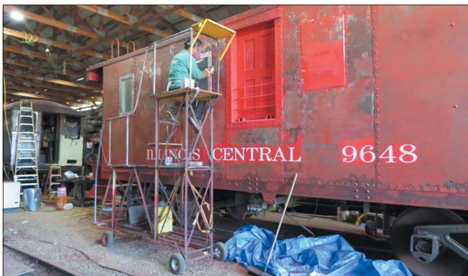
Thee is working to remove paint on May 30 th to bare metal so primer can be applied. The museum sand blasted the car when it was on the IC interchange when it arrived in 1993 so this is the second time the body is going to bare metal at the museum.
