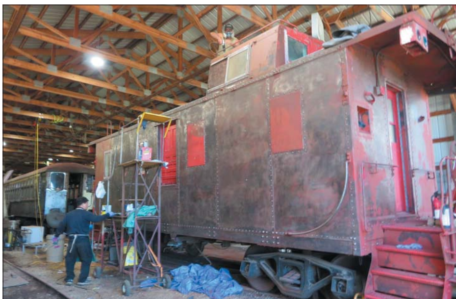
On June 13 th , 2021 we see how the needle scaling and sanding is progressing.
