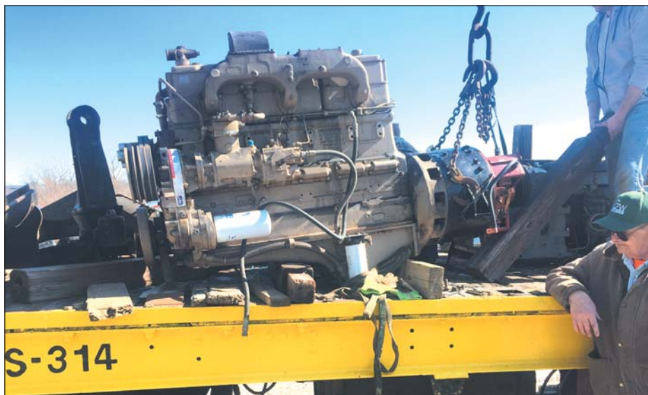
| The Cummins diesel and generator resting on S-314's deck before reinstallation.
