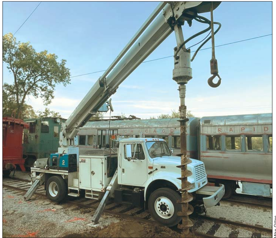
Jeff's high-rail auger truck drilled all the foundation footings.
