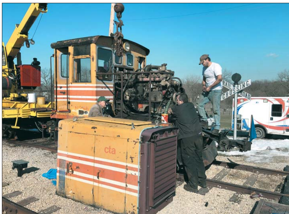
| The prime mover back on the locomotive on March 6 th , 2022. Mike Gilles photo
